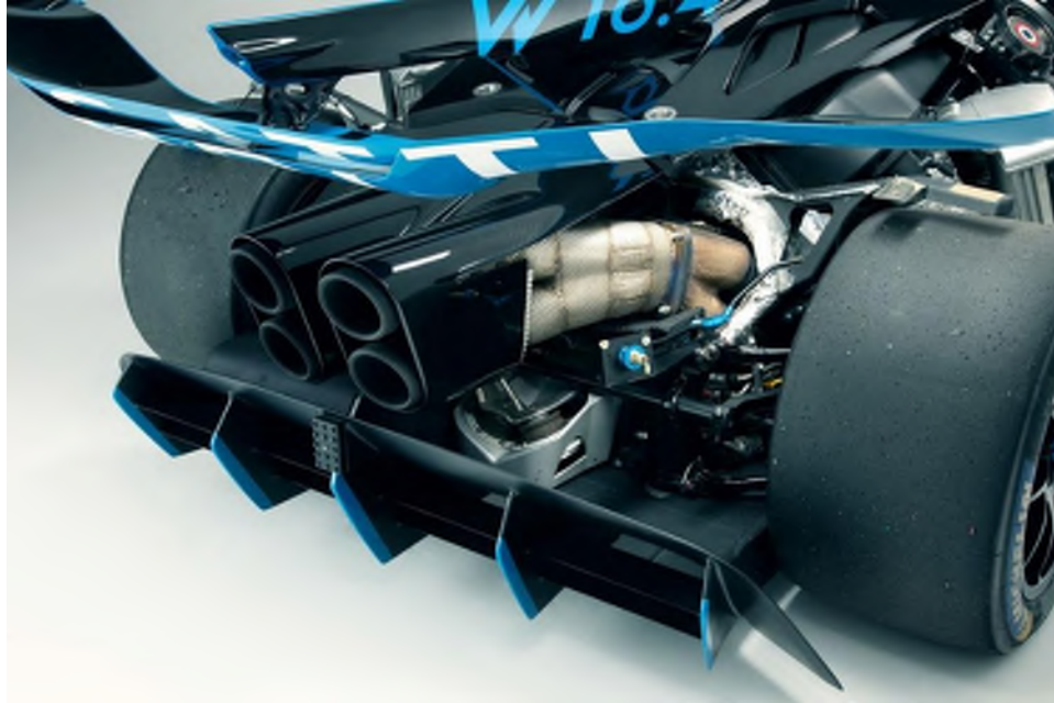
Photo 2 - 3D-printed titanium component that holds the rear wing
