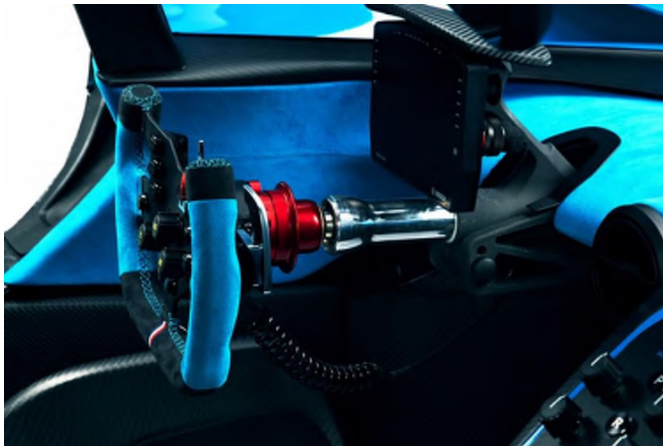
Photo 1 - 3D-printed titanium mounting brackets
