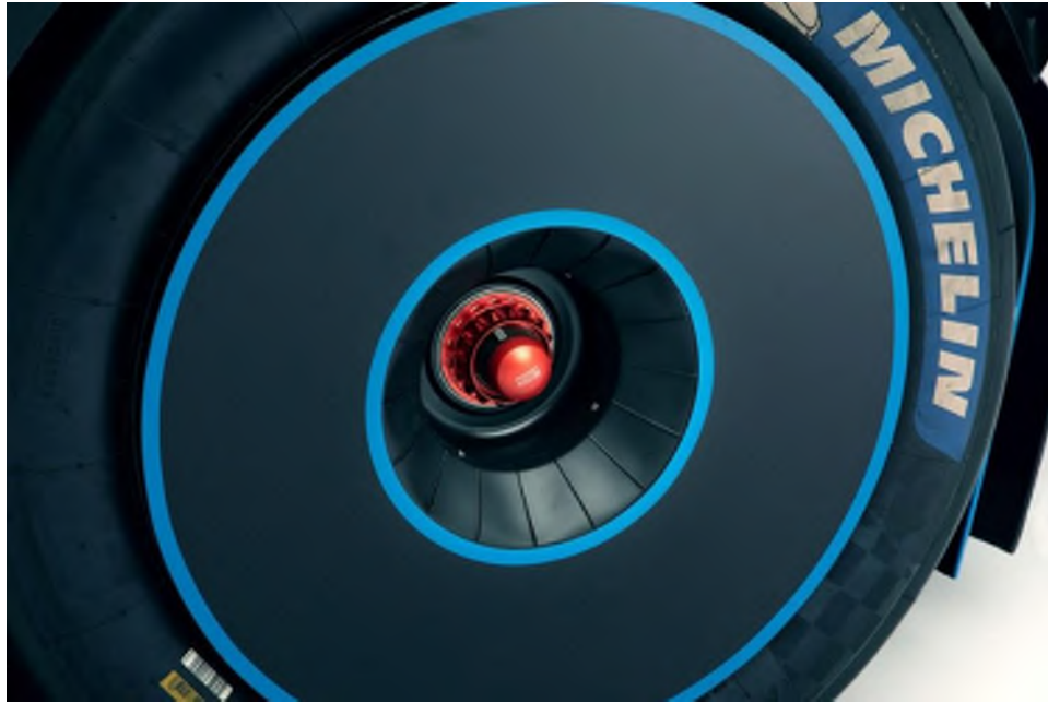
Photo 5 - 3D-printed wheel-mounted radial compressors
